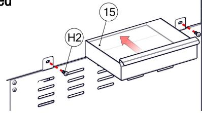
Align mounting holes of grilling chamber with cabinet slots.
