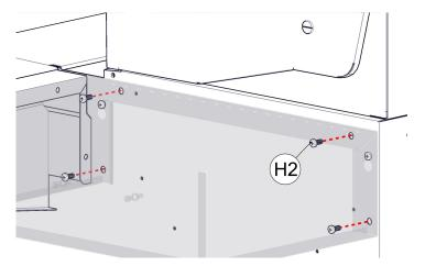
Secure shelf using 4x M6 Phillips Screws (H2) through the shelf body into the grill body. A screwdriver works best in this tight space.
