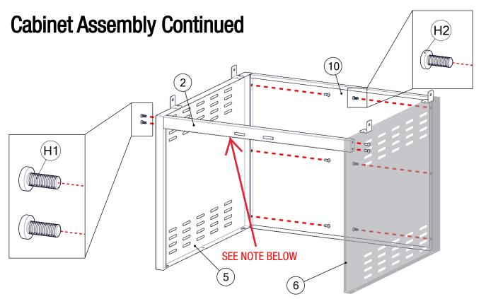
Assemble cabinet sides and back using 6x M6 Phillips Screws (H2). Attach cabinet front bracket to sides using 4x M5 Phillips Screws (H1). **NOTE:** The cabinet front bracket should be oriented with the magnetic catches towards the cabinet bottom.
