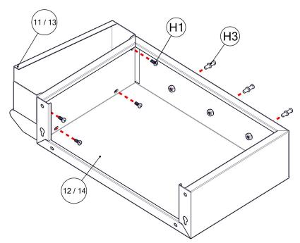
! Tighten screws carefully to avoid stripping out thread or Phillips drive!
