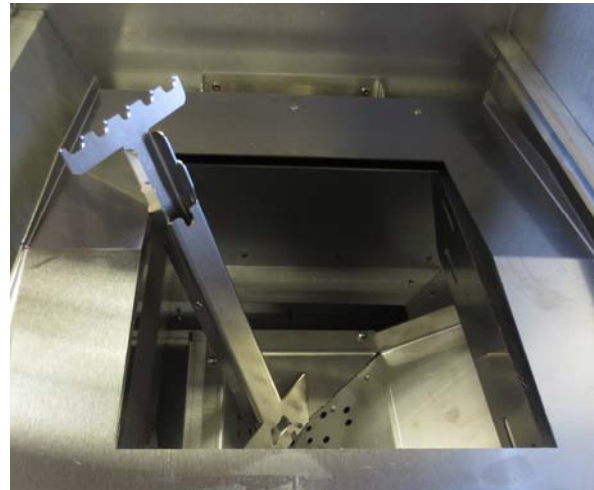
Step 3: Cleaning of the Burn Pot
